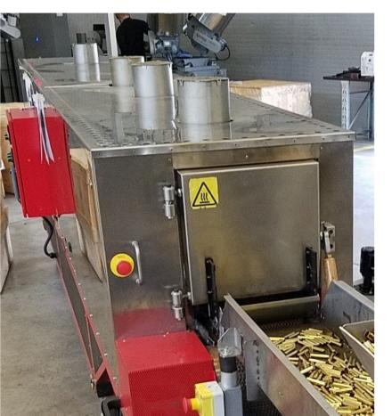
Annealing Unit is designed for strengthening of components to prepare them for drawing operations in case production. The tension of the metal conveyor is adjustable in order to prevent it from loosening because of expansion. The speed of the conveyor line and the temperature of the system are adjustable as well.
