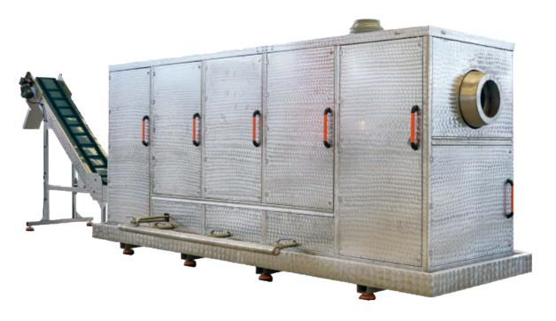
Degreasing Unit is designed to remove oil from semi- finished components. These components are exposed to oil in production presses and cannot be heated before degreasing process. It is a fully automated PLC controlled machine.
