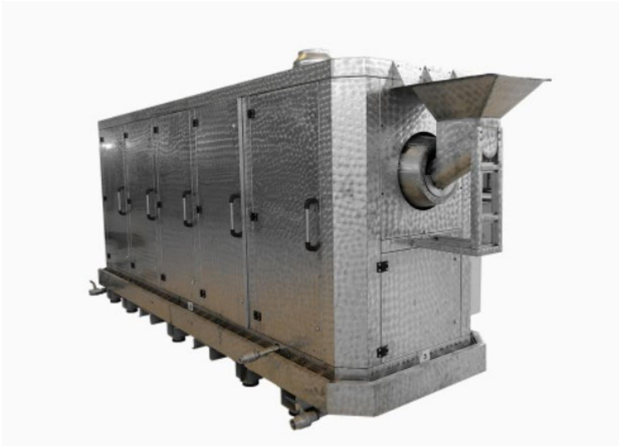
PICKLING UNIT Pickling unit is dedicated for washing semi-finished components by acid to remove oxidization created by annealing /normalization operations in previous machines.
